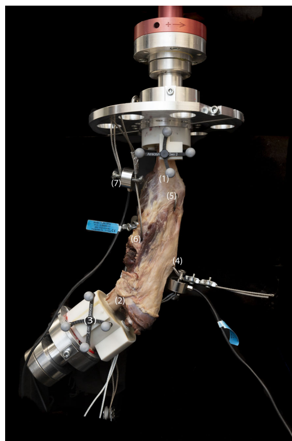
FIGURE 3 Experimental setup (right stifle; lateral view). The tibia is potted and aligned with the rotary axis of a linear–torsional testing system (Instron E3000) (1); the femur is potted and secured in a custom six-degree-of-freedom fixture (2). Reflective marker clusters on the femur and tibia (3) enable optical tracking (FusionTrack 500, 100 Hz) of internal tibial rotation (°) and cranio-caudal translation (CCT, mm). Muscle loads are applied by pneumatic actuators (off frame) and transmitted via stainless-steel cables routed along physiologic lines of action: Quadriceps via a mediolateral patellar tunnel (4), biceps femoris anchored at the tibial tuberosity with lateral 10–15° proximal angulation (5), and gastrocnemius routed caudal to the femoral condyles around the fabellae (6); inline load cells (7) monitor cable forces. The machine applies axial compression (30% bodyweight); a base-mounted shear actuator (not visible) applies cranio-caudal loading for CCT tests.
